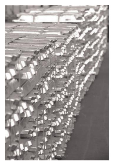
Sales of aluminum alloy ingots accounted for approximately 12.0%, 4.5%, 5.8% and 2.8% of our revenue for 2017, 2018 and the six months ended June 30, 2018 and 2019, respectively. Molten aluminum alloy is processed into aluminum alloy ingots through molding, casting and cooling. Our aluminum alloy ingots are produced by using self-manufactured molten aluminum alloy.
